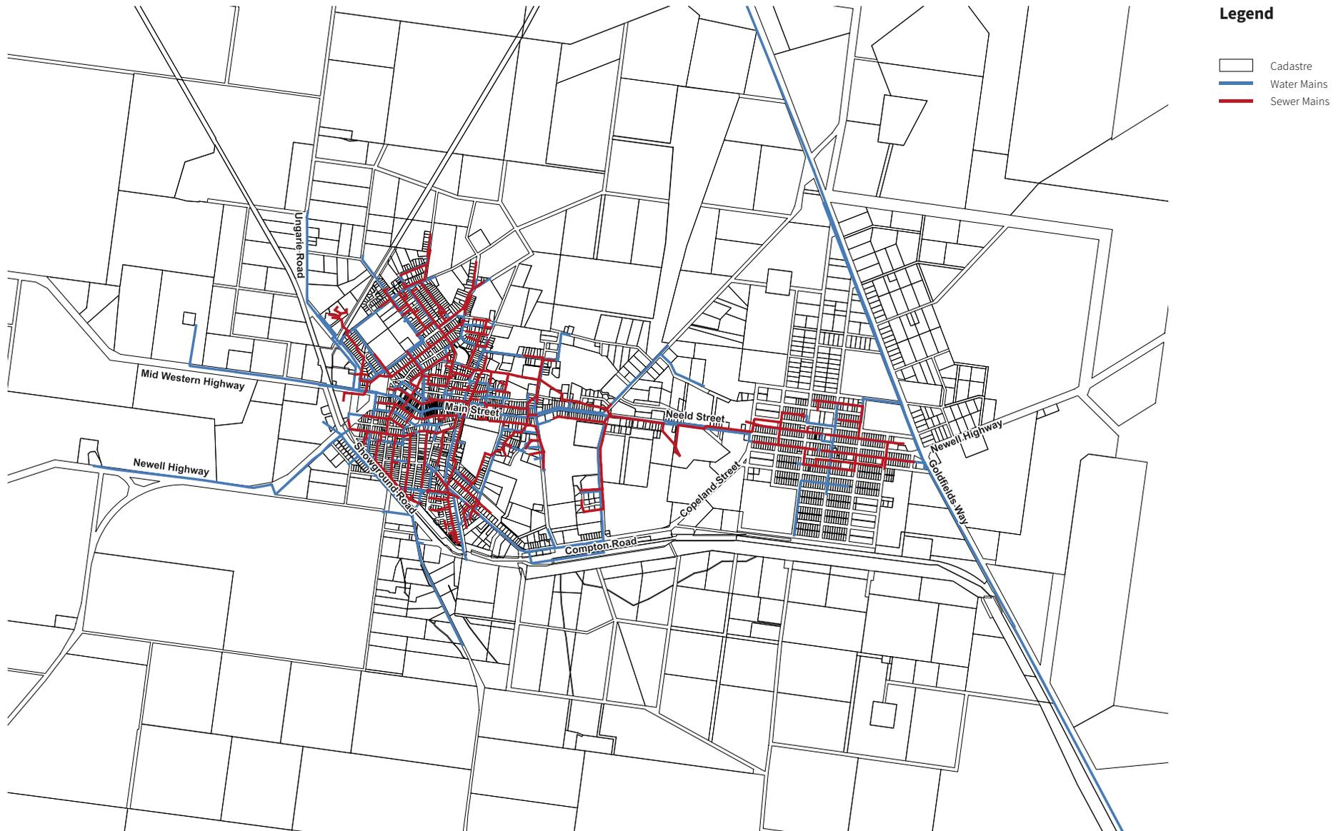
Figure 26: Water and Sewerage Infrastructure
